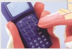
With trigger switches on both sides and large magic keys, it can be carried in many ways. While the body is compact, the key pitch is a wide 13.7 mm, enabling you to improve input speed. The keys are made of resin, so you don't have to worry about the letters disappearing.
